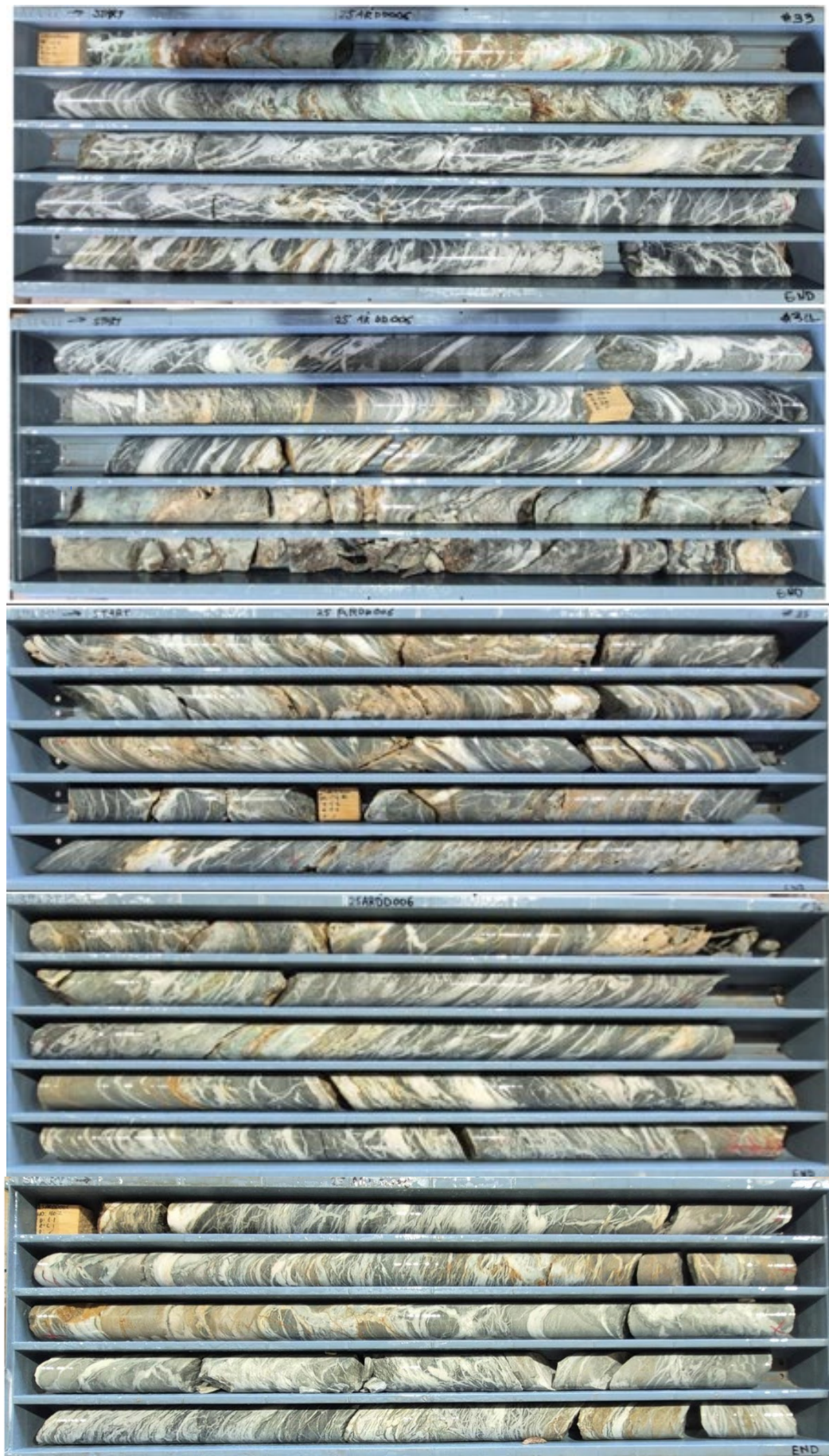
Figure 5: 25ARDD006 - drill core from 140.0-164.8m showing intensive quartz veining and related alteration within interpreted Titan East shear zone (assays pending)
