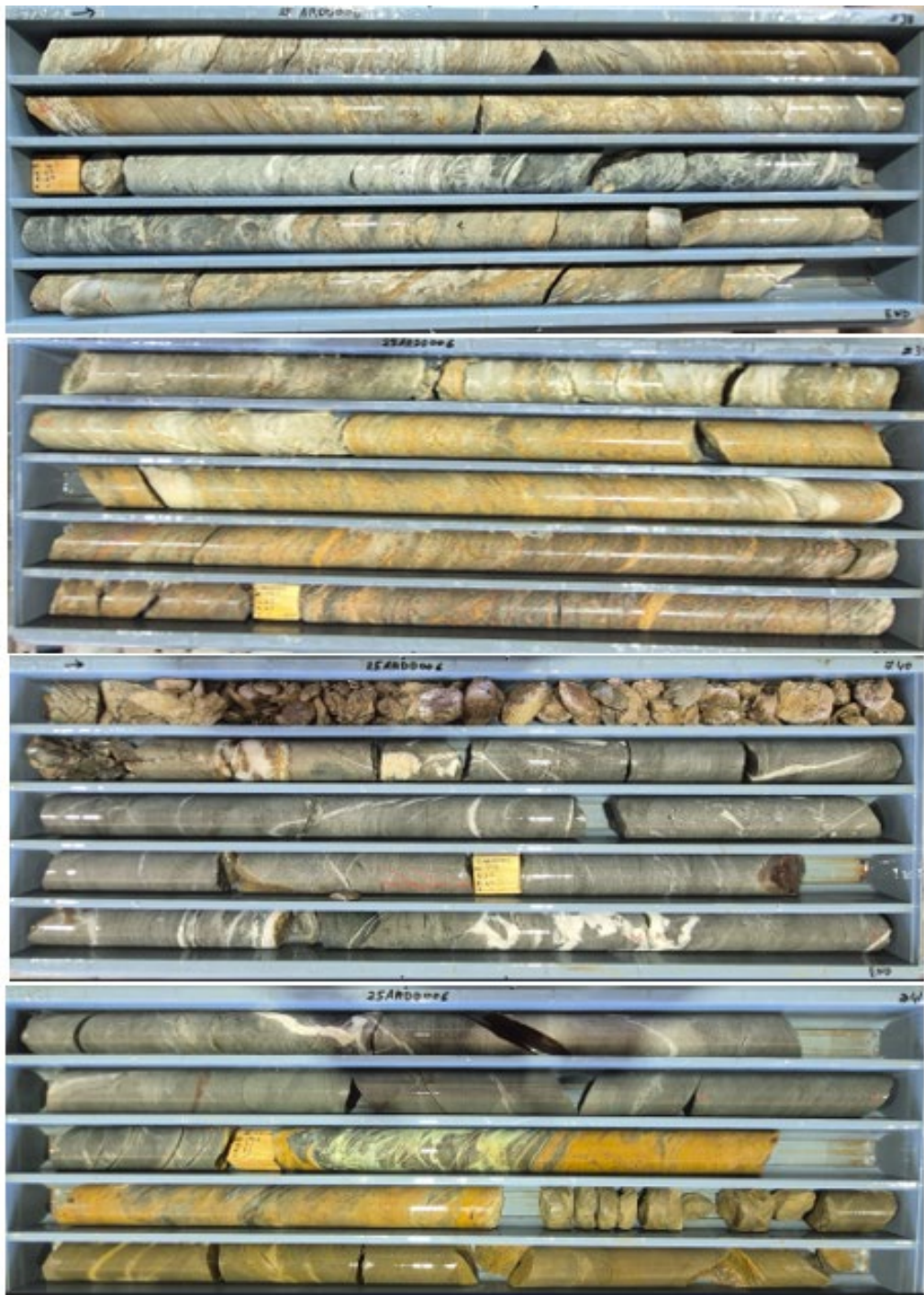
Figure 6: 25ARDD006 - drill core from 164.8-185.0m showing strong alteration associated with basal contact of interpreted Titan East shear zone (assays pending)
