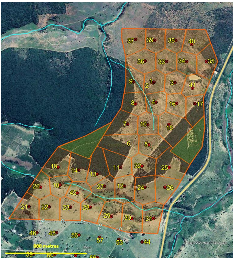
Figure 4. Irajuba IR-1 prospect polygons constructed in the drilled area of the Exploration target. Polygons were not constructed over the areas distant from drill holes that were not able to be drilled at present.
