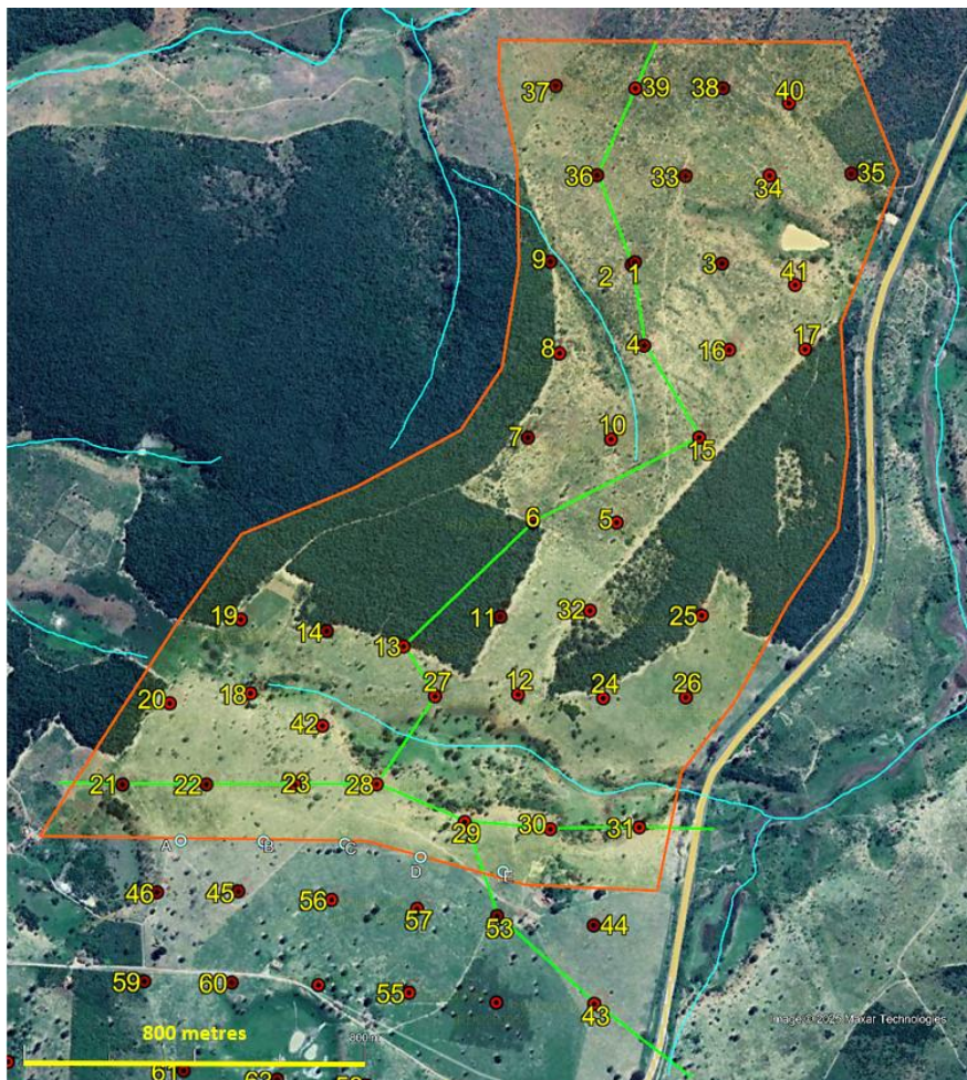
Figure 3. Drill sections (highlighted in green) which were designed to predominantly traverse along the major ridges while remaining centrally located within the Exploration Target area.
