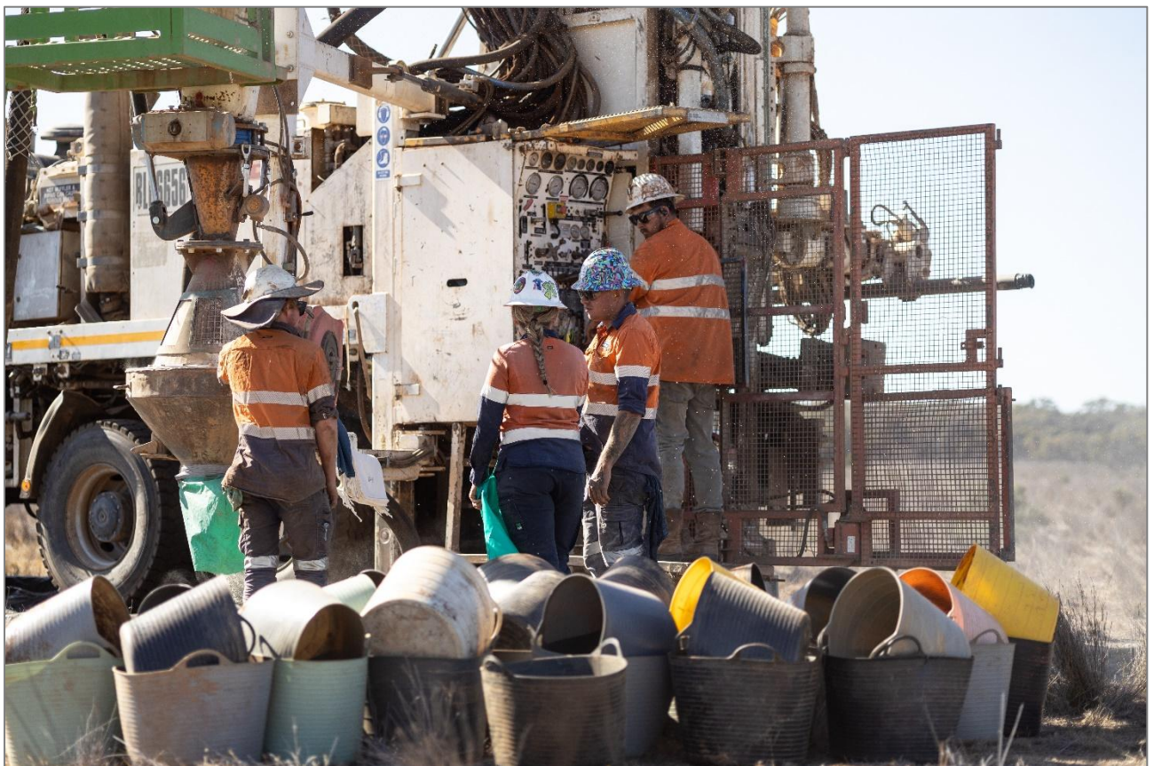
Figure 1: Air core drilling rig operating at the Murga Exploration Target December 2025.
