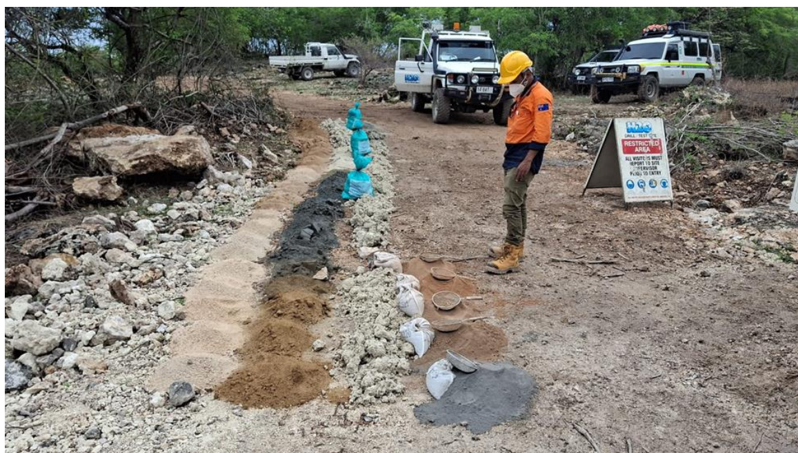
Figure 7: RC drill-cuttings from drill-hole WLR025 laid out in sequence.
