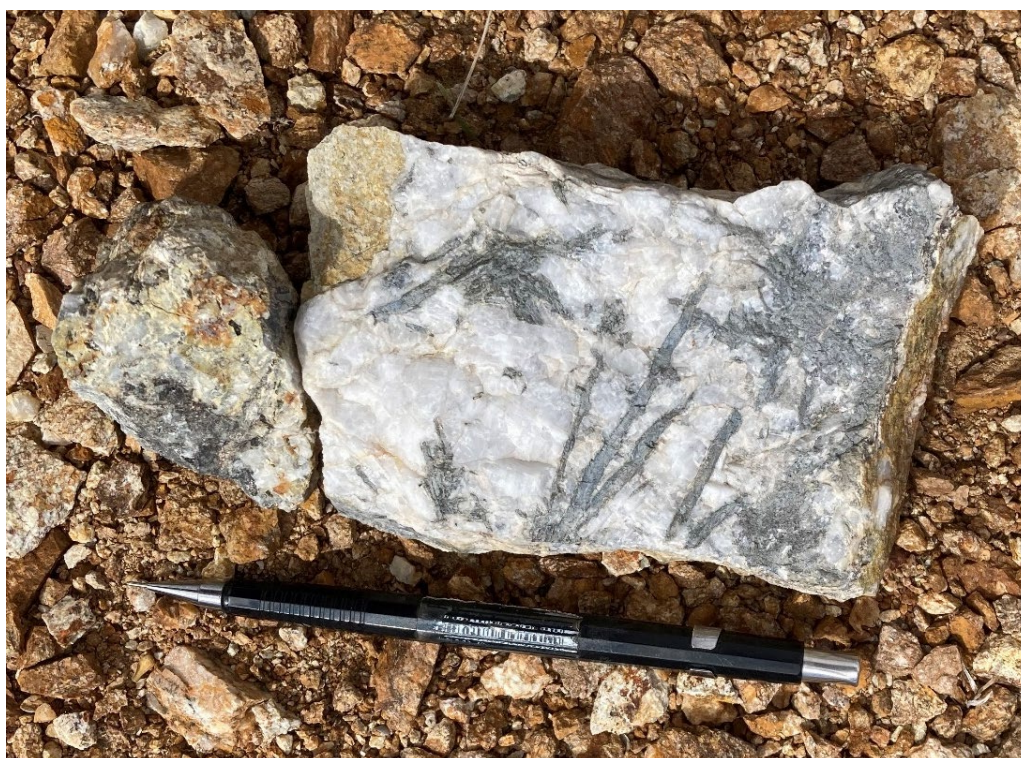
Figure 1: Photograph of Sample 258578 (see Table 1) from the Antimony Gulch adit which displays a quartz vein with approximately 8% coarse bladed stibnite (antimony sulphide) which assayed 6.16% antimony, 6.9 g/t silver.
