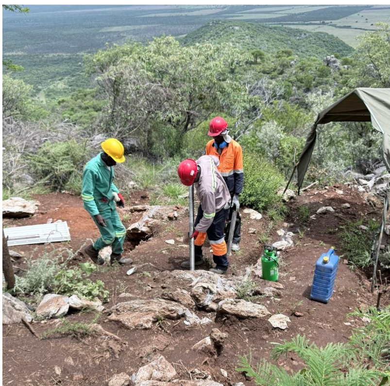
Images 2: Man-portable diamond rig testing Gossan 1 East. Image 3: Company personnel pulling rods with core enclosed
