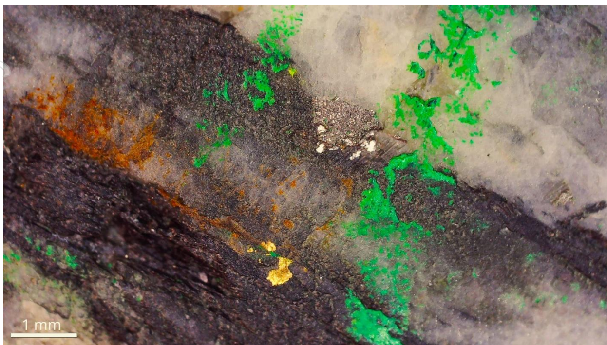
Figure 1: St Arnaud Comstock visible gold (25NED007 logging complete, assays pending) and pyrite. Note, the green colour is residual chinagraph pencil markings from the logging process.
