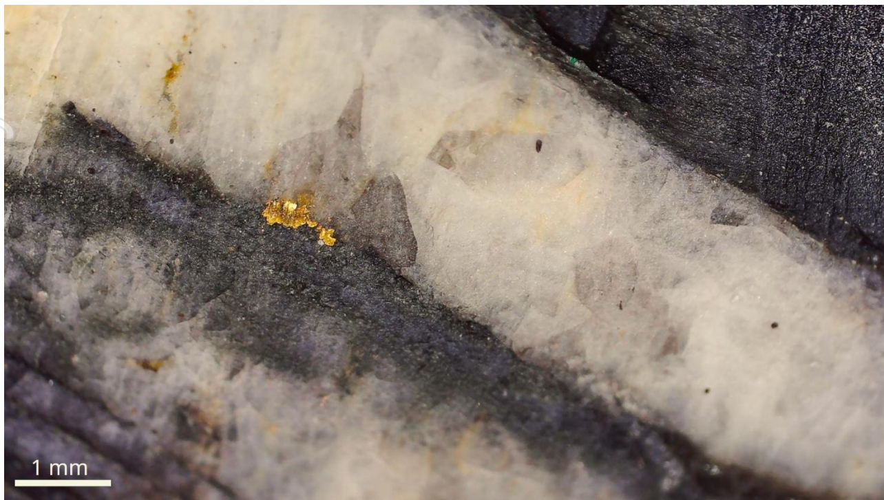
Figure 3: Microscope image of core containing visible gold 25NED007.
