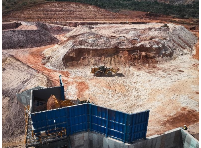
Figure 4: Ore Feed to Saprolite Crusher
