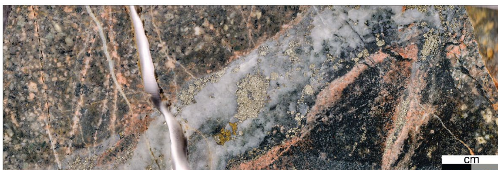
SPD013 67.3m quartz - pyrite - chalcopyrite - magnetite vein with potassic alteration selvage hosted in sodic altered quartz feldspar porphyry. 44.34 g/t Au.
