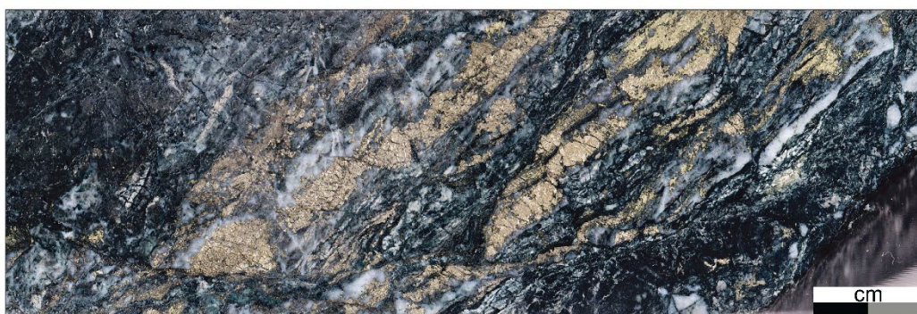
SPD012 275.9m Laminated quartz - pyrite ± feldspar ± chalcopyrite shear zone associated with high grade Mineralisation at Spur hosted in volcaniclastic sandstone. 19.81 g/t Au.
