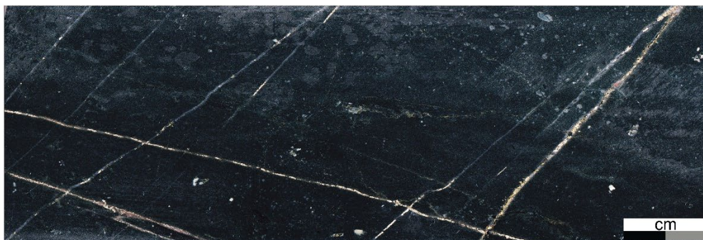
SPD013 157m quartz - pyrite and pyrite stringers in hosted in basalt. 5.88 g/t Au.
