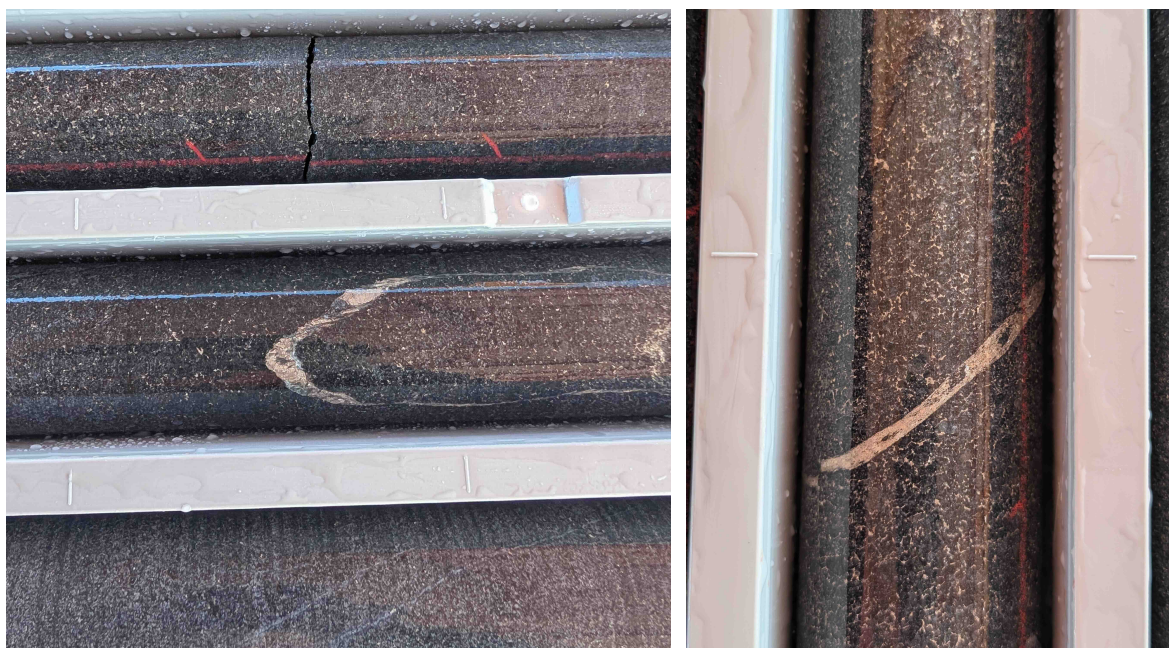
Figure 5: Photos showing examples of heavily disseminated sulphide in hole MTRC009 (EIS9) (top 1340m, left 1355m, right 1350m)
