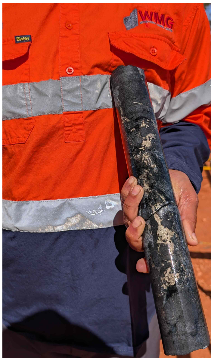
Figure 1: Photo showing example of sulphide segregations in hole MTRC009 (EIS9)
