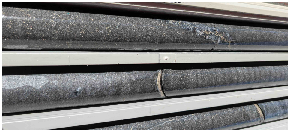
Figure 4: Photo showing examples of sulphide segregations in hole MTRC009 (EIS9) Note: core is NQ2 being 2 inches or 50mm diameter
