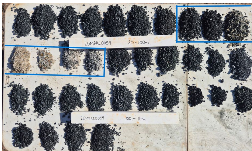
Figure 3: 25MPRC0059 drill chips showing a good intersection from 88m grading 10.65g/t gold over 7m
