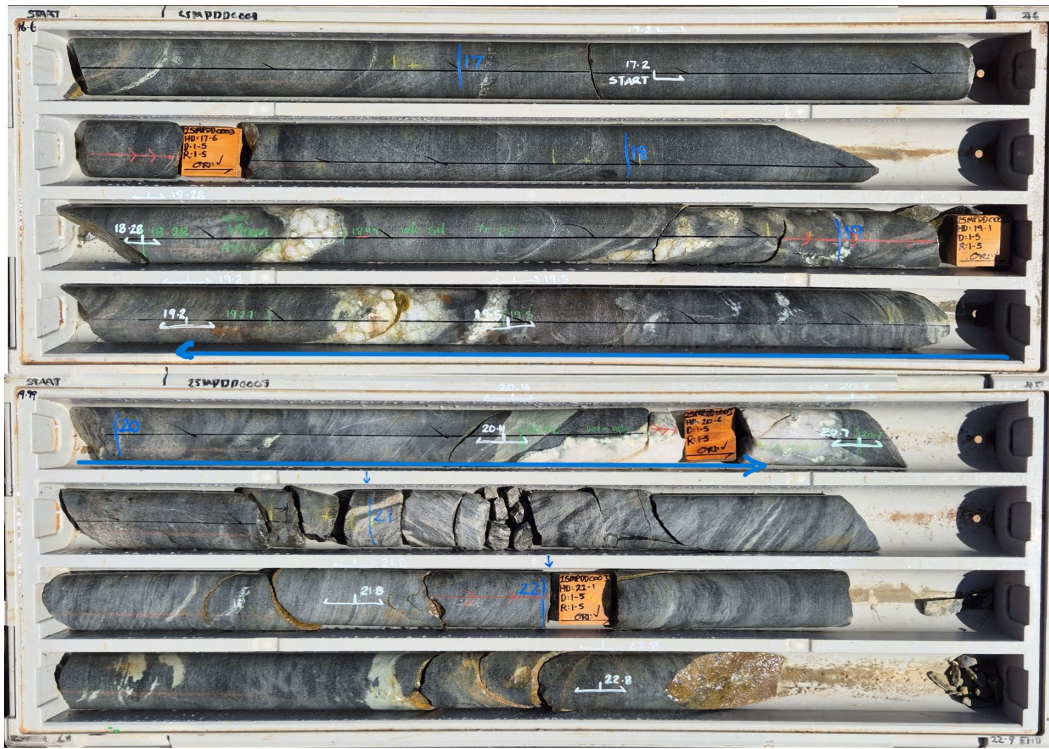
Figure 5: 25MPDD0003 core tray showing intersection of 1.2m @ 13.9g/t gold (from 19.2m) incl. 0.3m @ 54.5g/t gold (from 19.2m) (blue line showing the resulted zone)
