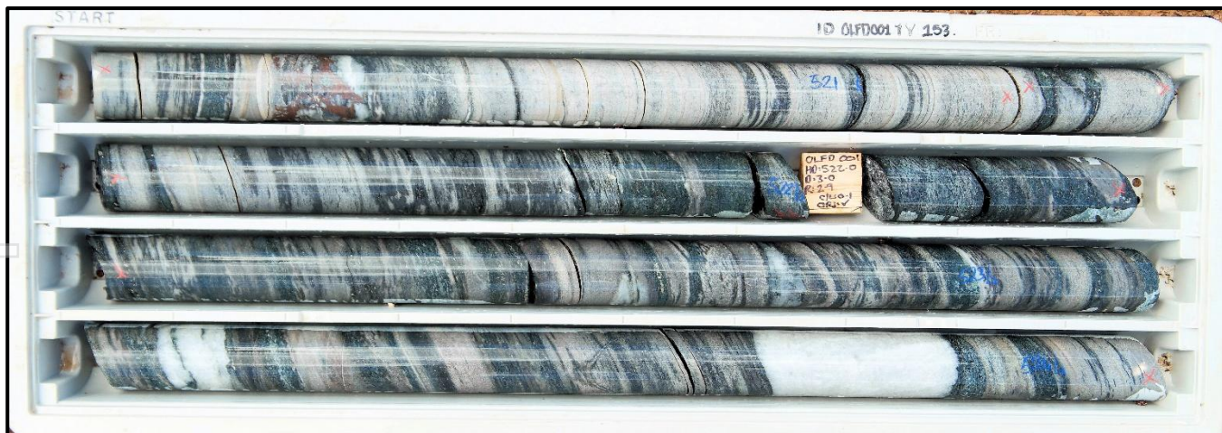
Figure 1 – Drill core from hole OLFD001 at Lennon's Find Project, from 520.3 to 524.1 metres downhole depth. Dark brown mineral is sphalerite (zinc sulphide) with galena, chalcopyrite and pyrite (refer Tables 1 & 2 overleaf) 1
