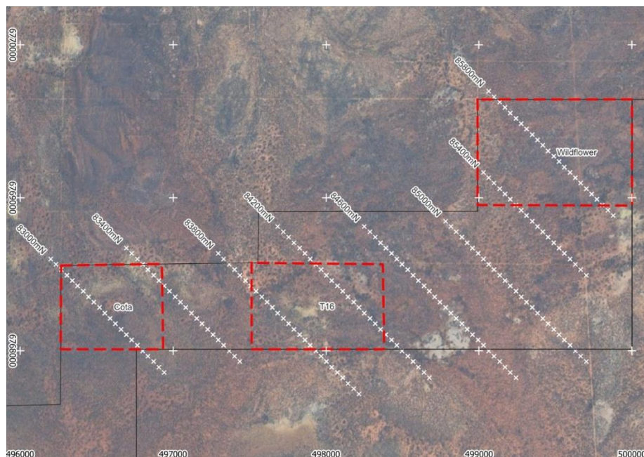
Diagram 11: Location of the induced polarisation (IP) survey stations and lines (shown in white) across Terrain Minerals Wildflower granted tenement E59/2234 and extending into Terrain Minerals adjoining granted exploration tenement E59/2345. The location of the three prospects within exploration tenement E59/2234, namely Wildflower (actual), T16 and Cota are outlined in red (see ASX release 10 November 2025).
