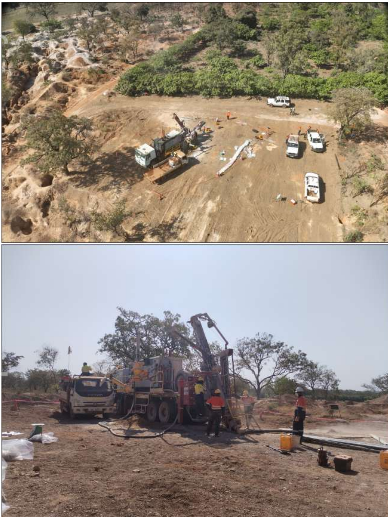
Figure 5: Sahara AC drill rig operating during Phase 2 strike extension drilling at Massan.
