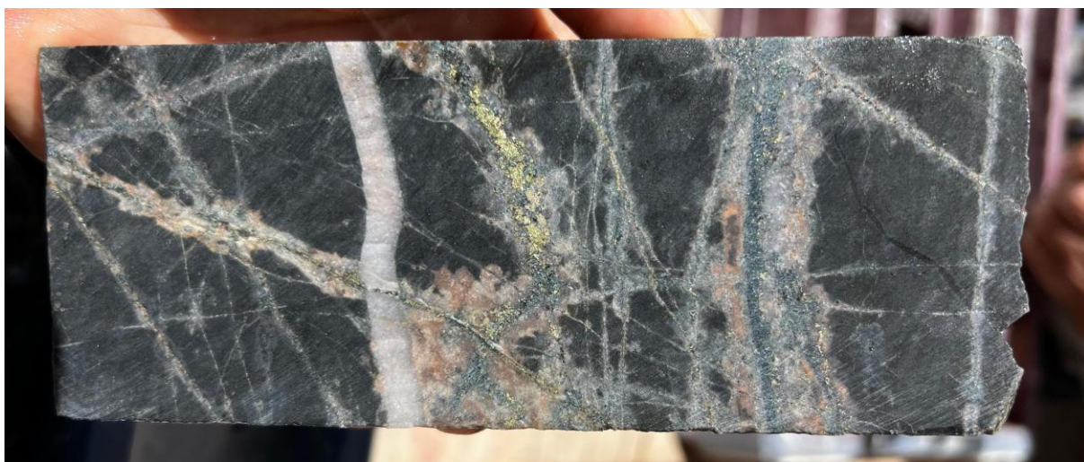
Figure 4: Core photo from CANDD002 at 379m, showing multiple vein sets within the host volcanics and quartz sericite veins containing chalcopyrite (brassy yellow colour).
