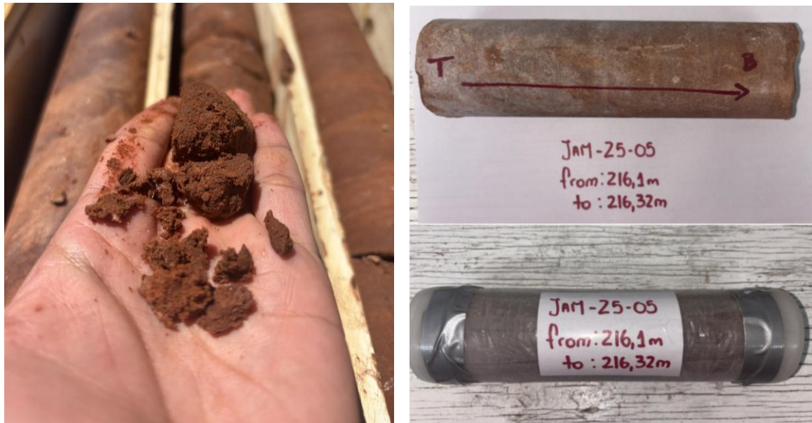
Figure 4. Core- fine wet sands in a clay matrix at 179m depth and cores sent for porosity analysis.
