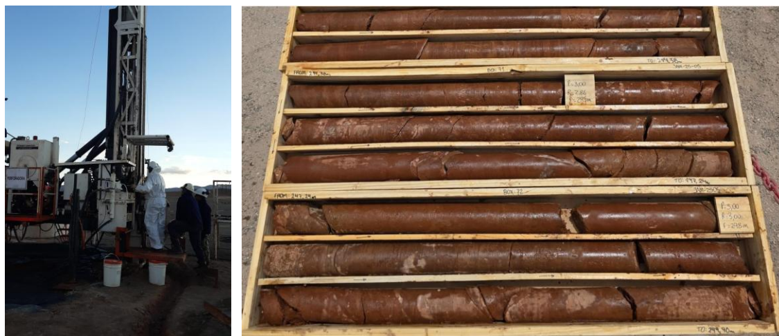
Figure 2. Well conditioning on 5 January and right hand side picture shows porous core at 241m with sand evident.
