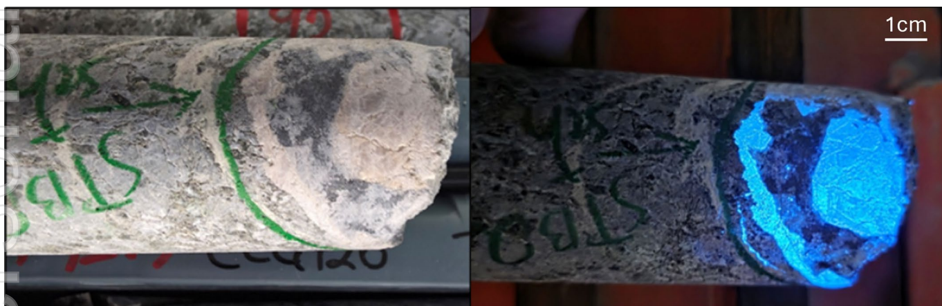
Figure 6: Scheelite (tungsten) mineralisation in CLG126 diamond drill core. Fluorescence observed under UV light.
