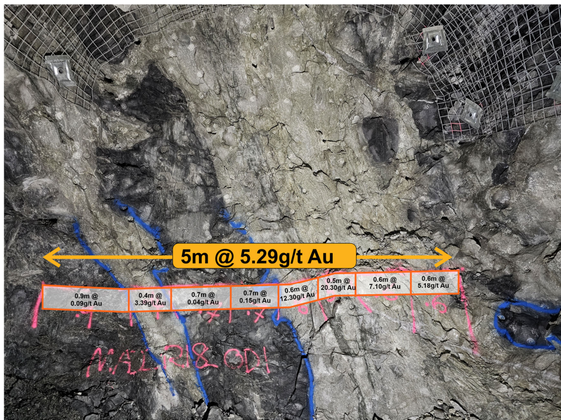
Figure 5: Photo of a development face on the 1281 OD1 showing sample grades and uncut weighted face average grade.
