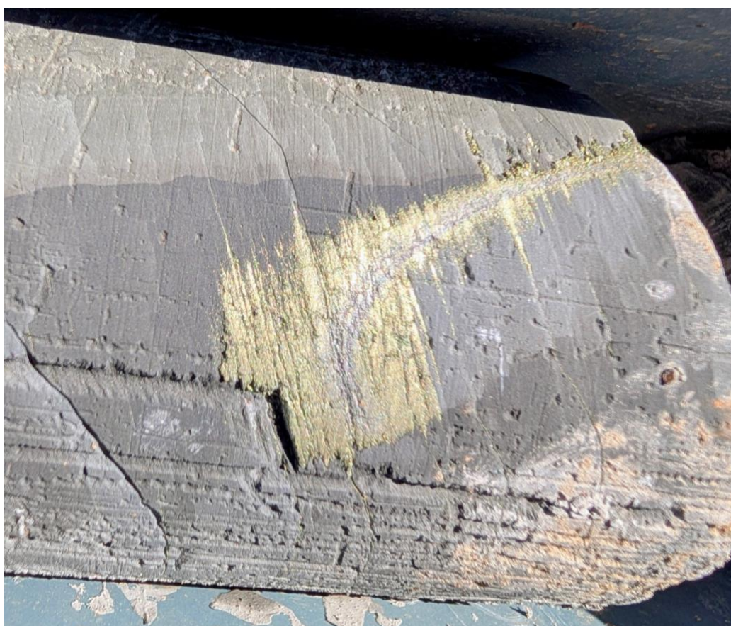
Figure 2 Tapley Hill Formation PQ drill core (85mm diameter) from the Windabout deposit, approx. 64.1m, DD25WIND0004. Sulphide abundance is estimated at approx. 50% chalcopyrite, 15% carrollite and 5% chalcocite in line with AIG guidelines. Note that these abundances are restricted to the immediate vein and are not representative of the broader intercept.
