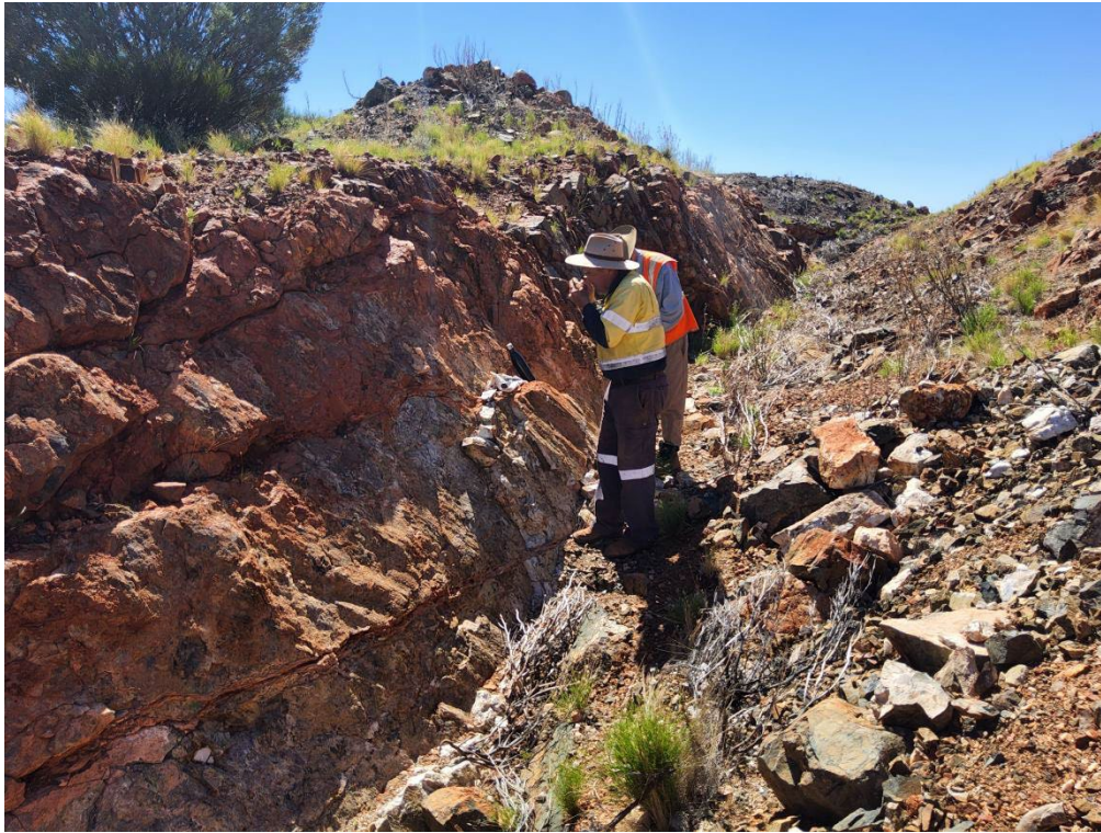
Figure 17. Kilkenny Workings – Field photograph showing historical costean, north wall oriented E-W, looking east, exposed sheared mafic rocks with quartz veinlets observed in sheared mafic rocks. Geological observation only; no assays are associated with this photograph. (MGA94 Z51 - 386600mE 6792215mN)
