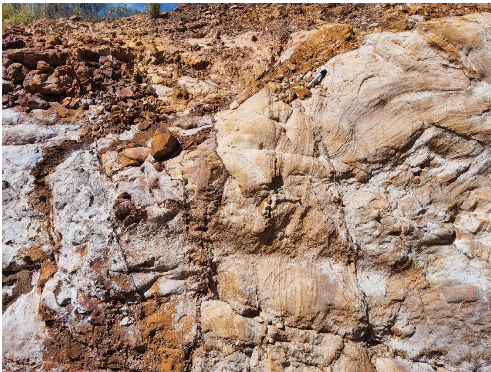
Figure 13. Ian's Reward prospect (tenement pending) – Field photograph showing quartz veining and associated alteration within host mafic lithology. Geological observation only; no assays are associated with this photograph. (MGA94 Z51 – 393782mE, 6794947mN)
