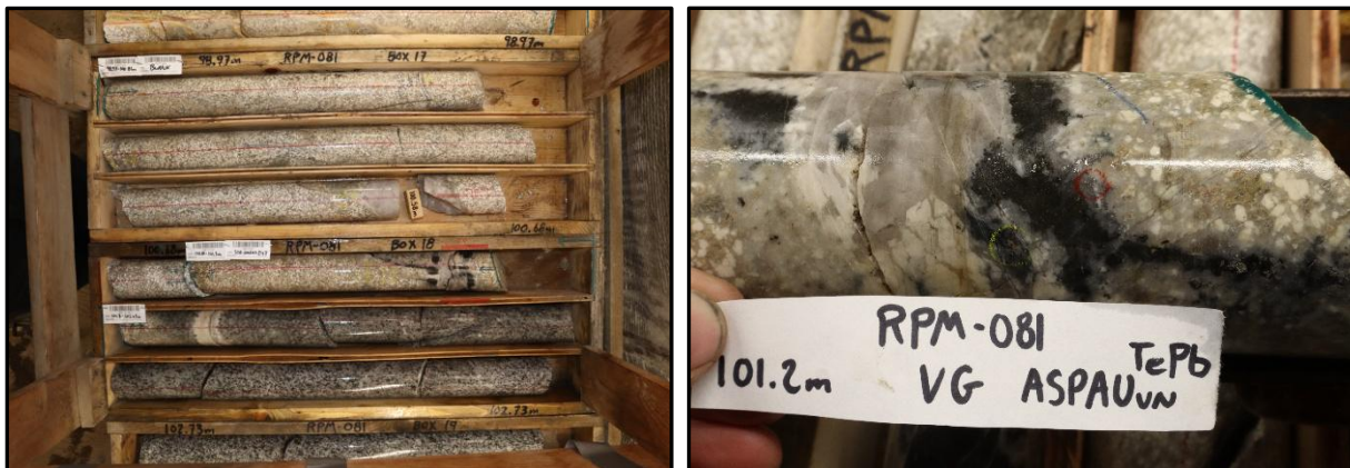
Figure 2. RPM Valley hole RPM-081 0.5m @ 364.0 g/t Au at 101m, with visible gold observed in the assayed core
