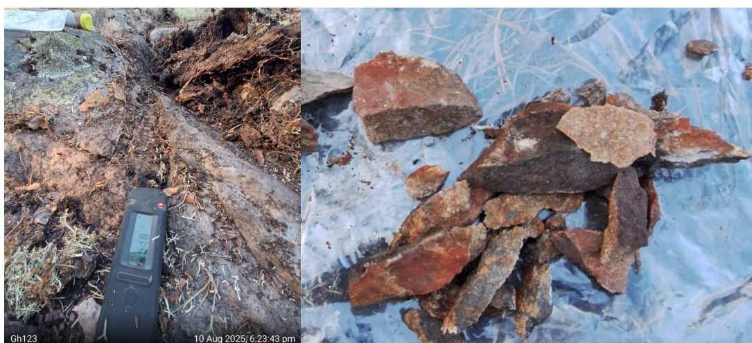
Figure 1: (left) Photograph of 20cm wide zone of shear-hosted uranium mineralisation and hematite alteration extending to the north where sample GH123 was taken & assayed 0.3% U_3O_8 ; (right) Close up photograph of hematite-altered rock samples GH123
