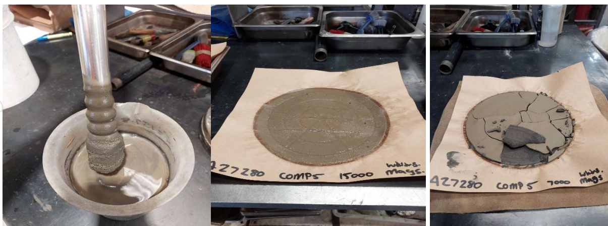
Figure 2: Eclipse Samples Being Prepared for High-Intensity Magnetic Separation Test Work (15,000 and 7,000 Gauss)
