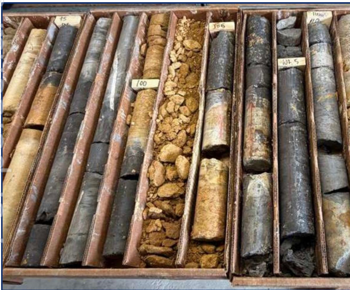
Figure 1 – Hole ACP26DD001 - Main mineralised horizon located between 95 and 110 feet downhole. The black mineral is massive to semi-massive stibnite, with an estimated abundance of 12% \text{Sb}_2\text{S}_3 . The main mineralised zone rests on a less mineralised conglomerate.
