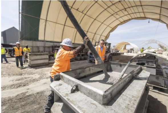
Figure 3 & 4: Wind farm concrete trials - 50% AusPozz™ mix design
