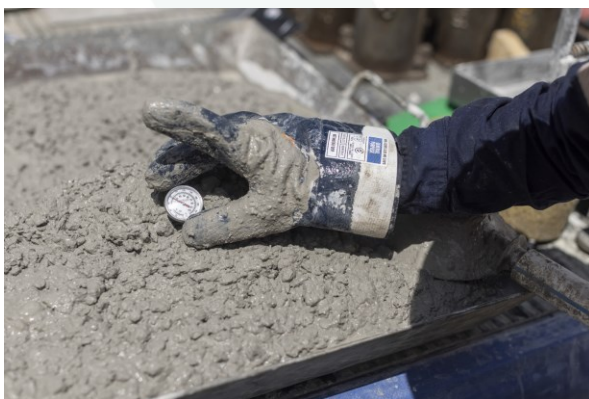
Figure 1 & 2: Wind farm concrete trials - 50% AusPozz™ mix design
