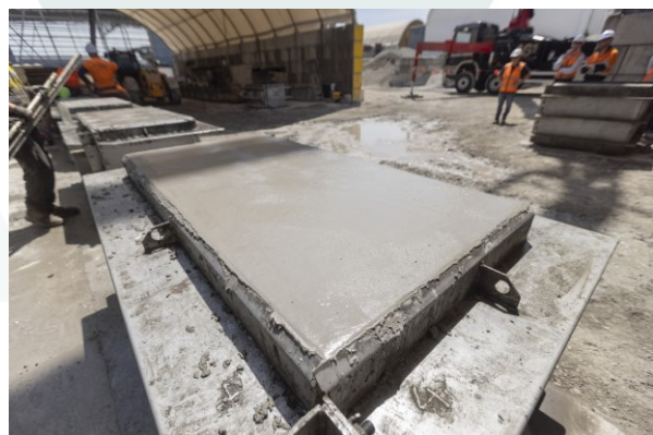
Figure 1 & 2: Wind farm concrete trials - 50% AusPozz™ mix design
