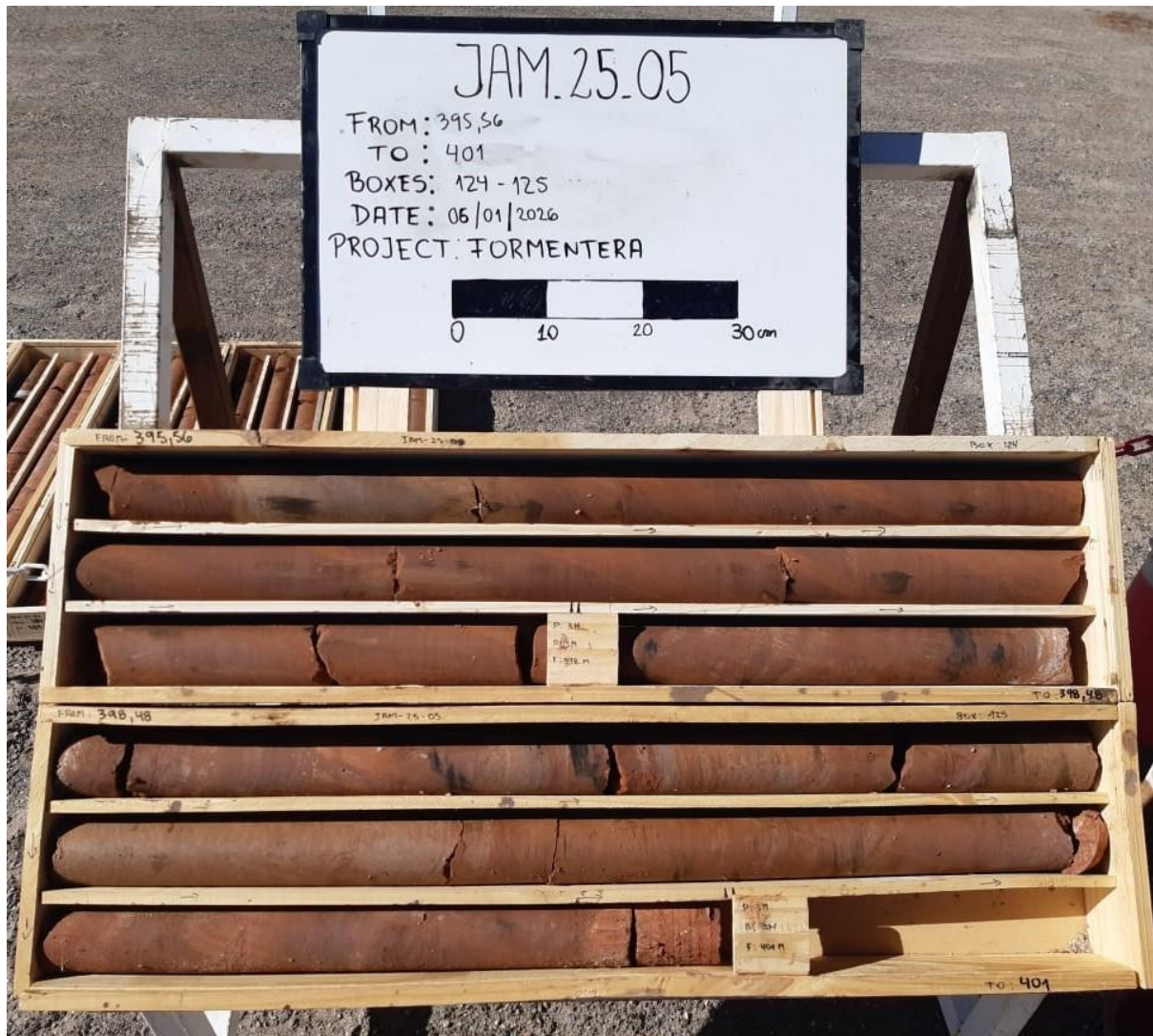
Figure 3. Final drill tray showing fine grained consolidated clays. Smectite is a very conductive clay.
