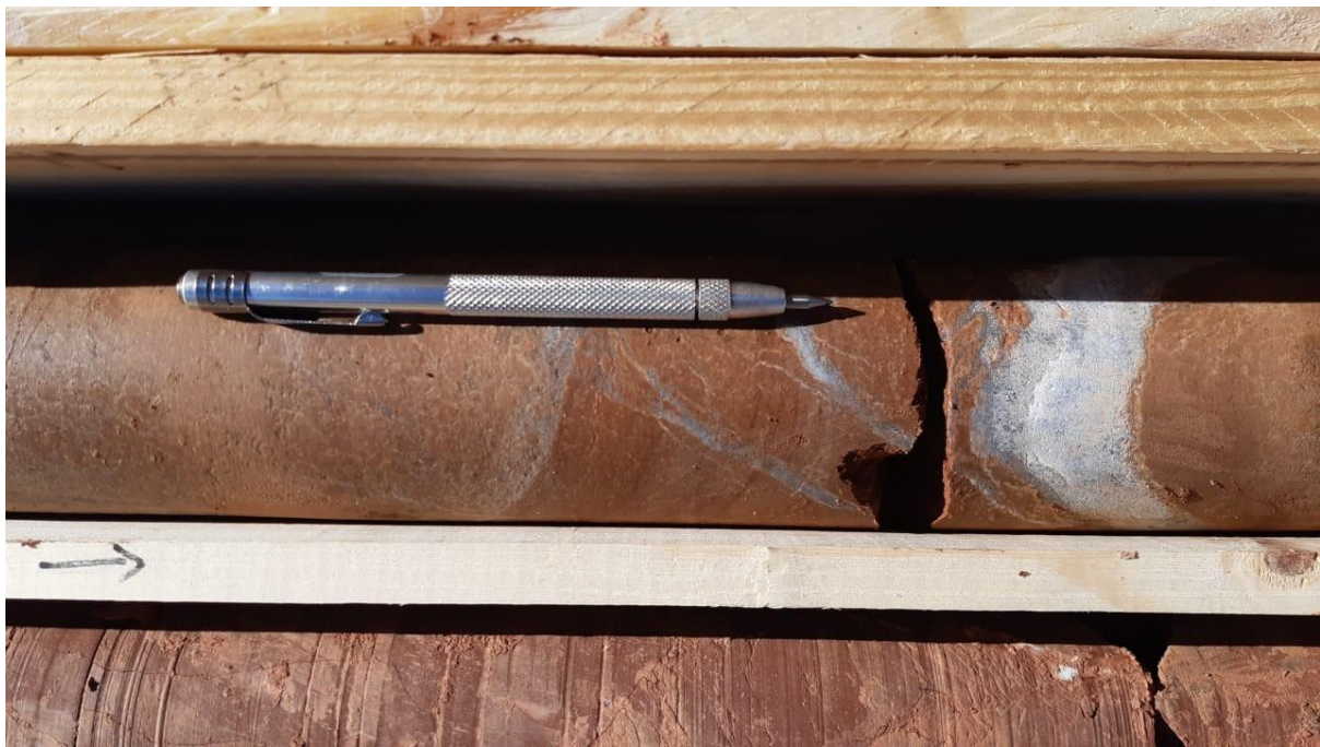
Figure 4. Shows fractures and veinlets infilled with gypsum/anhydrite ( \text{Ca}_2\text{SO}_4 ) in the clayey siltstone and appears to be a secondary event of calcium rich solutions precipitating in the veinlets.
