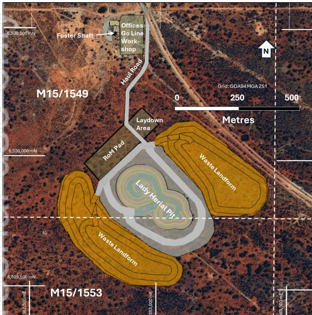
**Figure 13:** Lady Herial development and open pit mine design layout.
