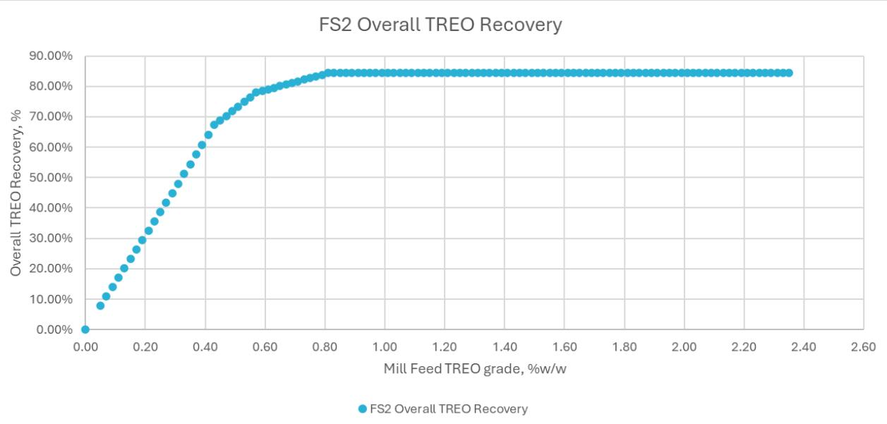
**Figure 2: Wolverine model of overall TREO recovery vs. TREO feed grade.**
