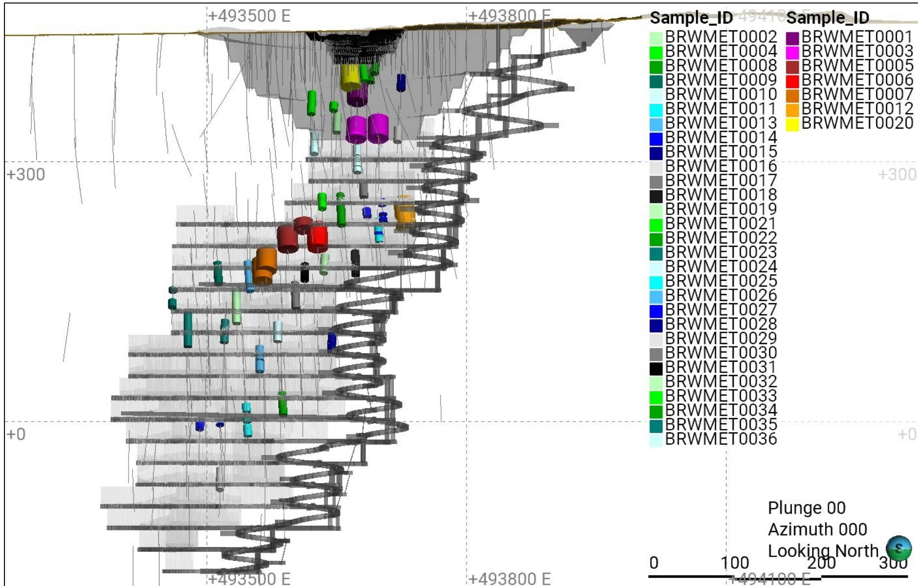
Figure 6: North-facing long-section of Wolverine diamond core metallurgical variability sample showing the Wolverine trial pit (black), and the DFS pit, box cut, development, and production designs in grey (ASX announcement 15 September 2025).
