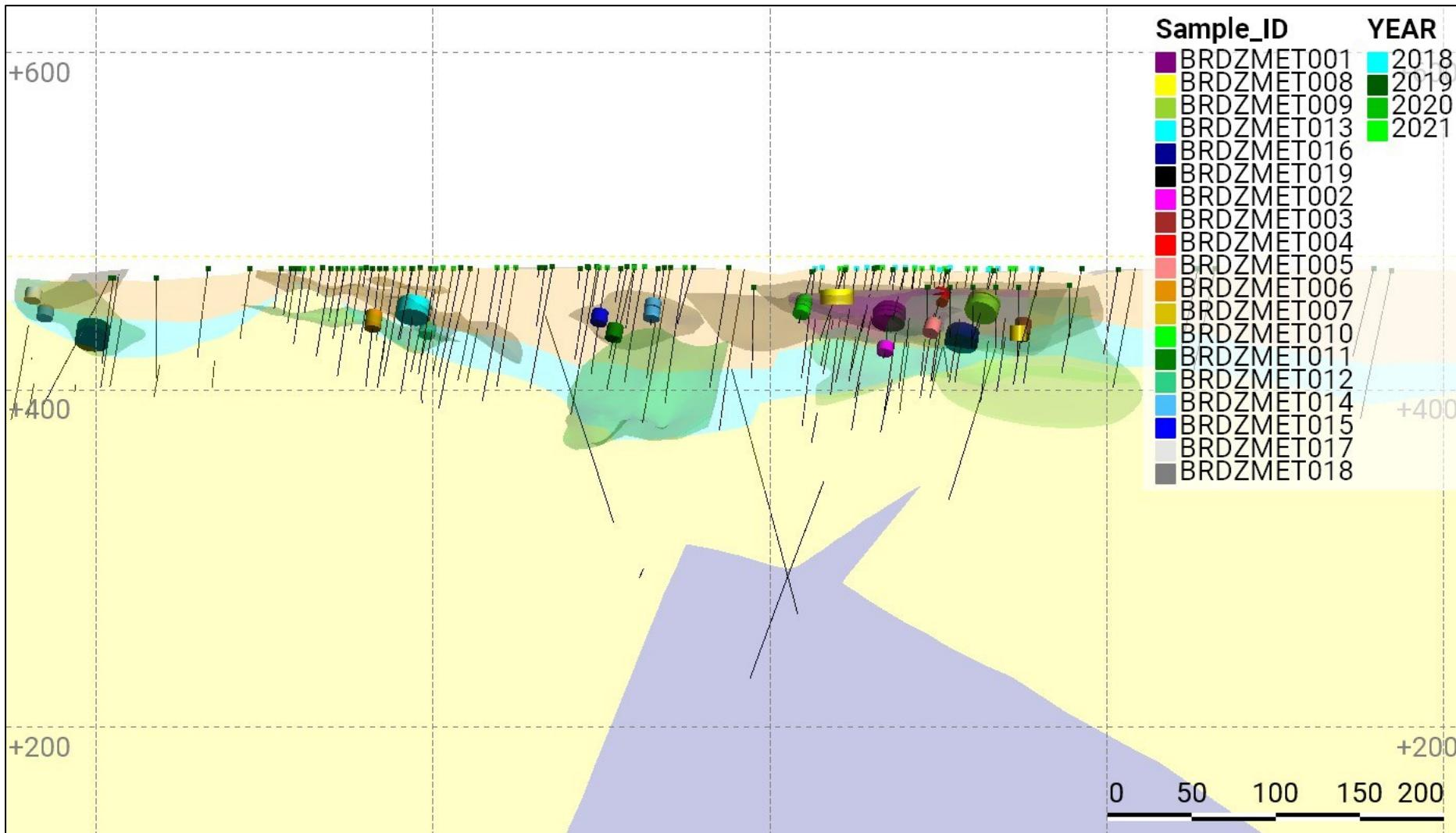
**Figure 4: NW-facing 75 m long-section of Dazzler metallurgical sample locations with composite IDs, the six Wolverine - Dazzler blend composites thicker, showing the 3D mineralisation model update and 2025 geological model (ASX announcement 13 May 2025).**
