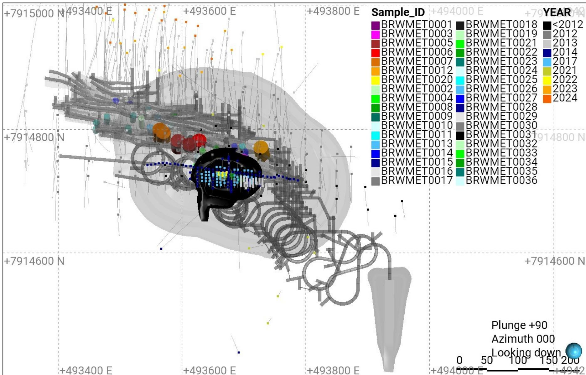
Figure 5: Plan view of Wolverine diamond core metallurgical variability sample showing the Wolverine trial pit (black), and the DFS pit, box cut, development, and production designs in grey (ASX announcement 15 September 2025).
