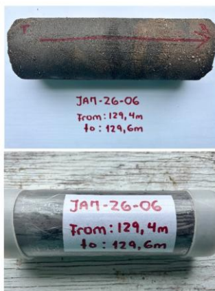
Figure 1. Core extracted at 129.4m ready for porosity testing and bottles of brine from Packer test ready for assay.
