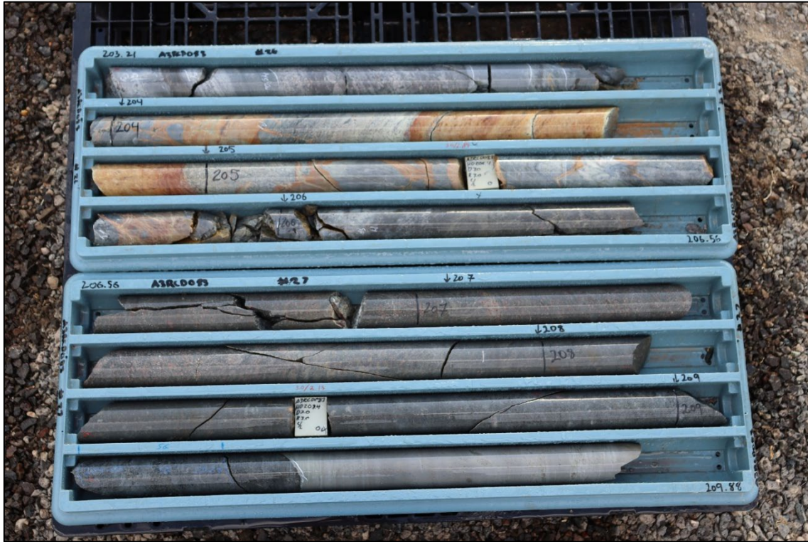
Figure 1: Core photographs of the gold-silver bearing zone in A3RCD083 grading 9.5g/t Au, 227g/t Ag; 1,123g/t AgEq over 3m from 205m to 208m. This high-grade interval occurs at the contact at 206.1m of the thinly bedded facies (upper) and dacite (lower).
