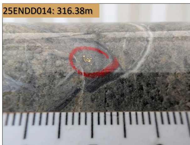
Left. Visible gold (circled red) in hole 25ENDD014 at 316.38m down hole in a quartz- carbonate-pyrite-arsenian pyrite vein within strongly phyllic altered granite host rock. Small ticks on scale bar are millimetres.
