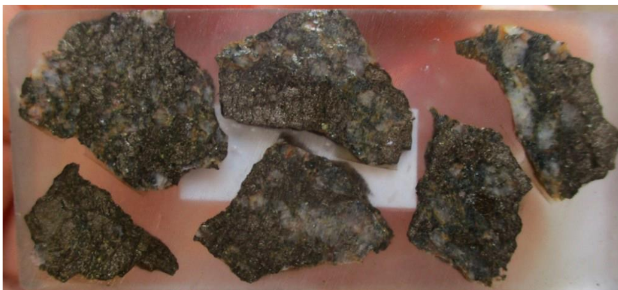
Figure 6: Sample 41 of appendix B ASX: PMM 01/12/2025 shows the clastic material in this sample is composed of transparent medium-grained quartz, small, black-coloured flakes interpreted as biotite, and light orange to pink-coloured blocky scheelite grains. These clasts sit within a matrix composed entirely of pyrrhotite.
