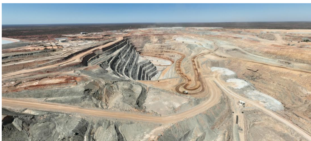
Figure 6: KoTH open pit, demonstrating tight working areas in the bottom of stage 1 as stage 2 is established
