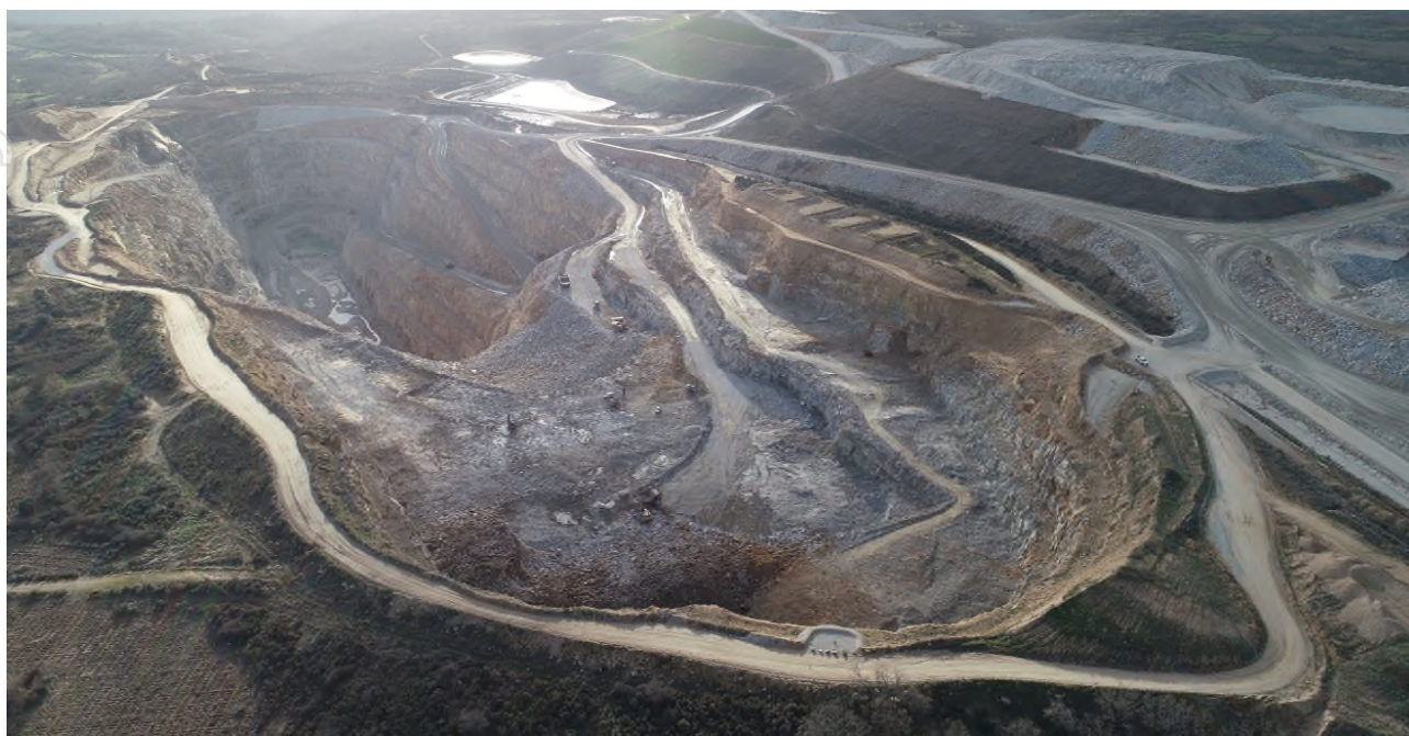
Pictured: Northern area of Phase 6 at elevation 680 RL, including the access ramp and the 670 RL bench.
