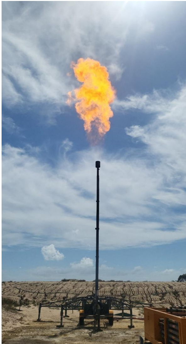
Wombat-5 gas flare on 19 January 2026, following blowing down with Nitrogen
