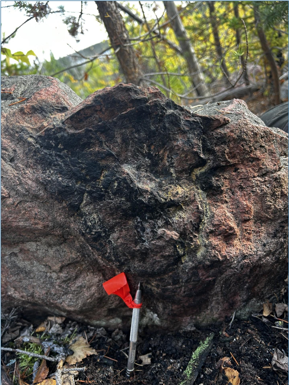
Figure 4: Identification of visible disseminated uraninite 1 showing at Reitenbach Lake (sample site 25RNB083, 623459E, 6423998N, UTM Zone 13). Rock chip assay results of the sample have since confirmed a grade of 1.90% U_3O_8 .
