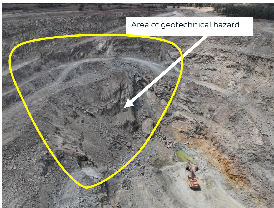
Figure 2: Pearce South open pit (looking north) showing geotechnical hazard region.
