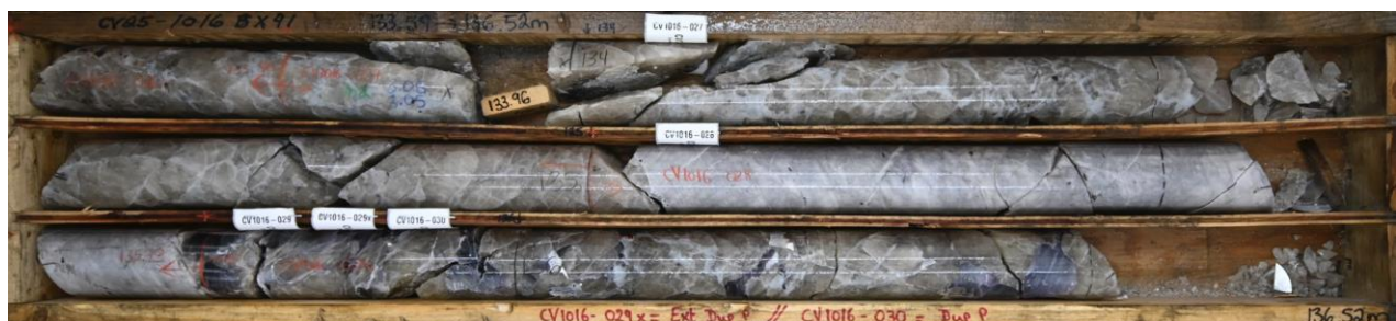
Figure 2: Massive spodumene in drill hole CV25-1016 from the Vega Zone at the CV13 Pegmatite. Core grades 0.7 m at 7.71% \text{Li}_2\text{O} (from 135.0 m to 135.7 m) within a wider mineralized interval of 49.7 m at 2.08% \text{Li}_2\text{O} (119.4 m to 169.1 m). At 7.71% \text{Li}_2\text{O} , this is the highest grade of lithium returned from an individual core sample collected to date at the Property.
