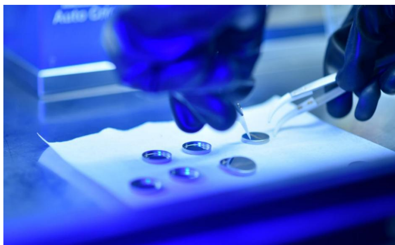
Figure 1: LMFP coin-cell batteries incorporating Firebird's proprietary battery materials.
