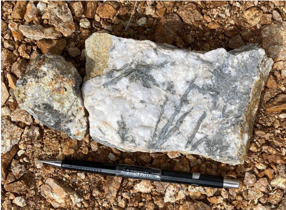
Figure 2: Photograph of Sample 258578 (see Table 1) from the Antimony Gulch adit which displays a quartz vein with approximately 8% coarse bladed stibnite (antimony sulphide) which assayed 6.16% antimony, 6.9 g/t silver.
