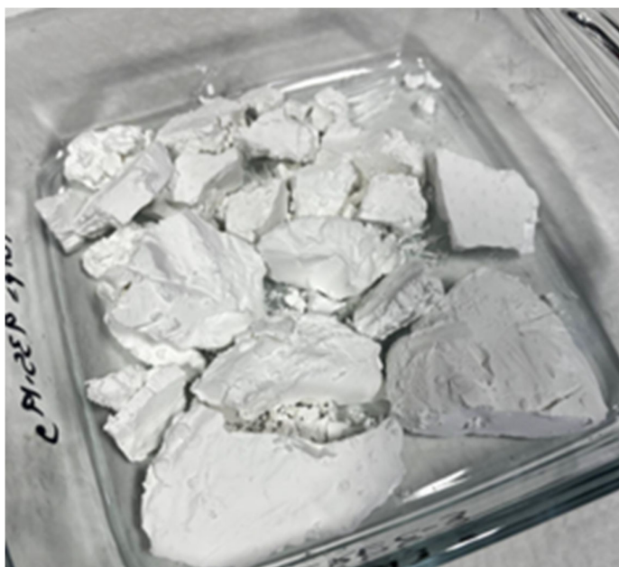
Picture 9. High-grade mixed rare earth carbonate (MREC) produced from Kangankunde monazite concentrate during ANSTO testwork, dense, low-radionuclide product suitable for downstream separation
