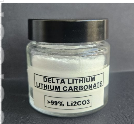
Figure 3: Mt Ida Lithium Carbonate produced from mica concentrate
