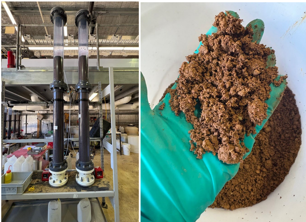
Figure 1: (left) Column leach tests in progress at ANSTO on 26 kg samples from the ABx Deep Leads deposit; (right) Post-leach clay from column C2 showing stability of agglomerates
