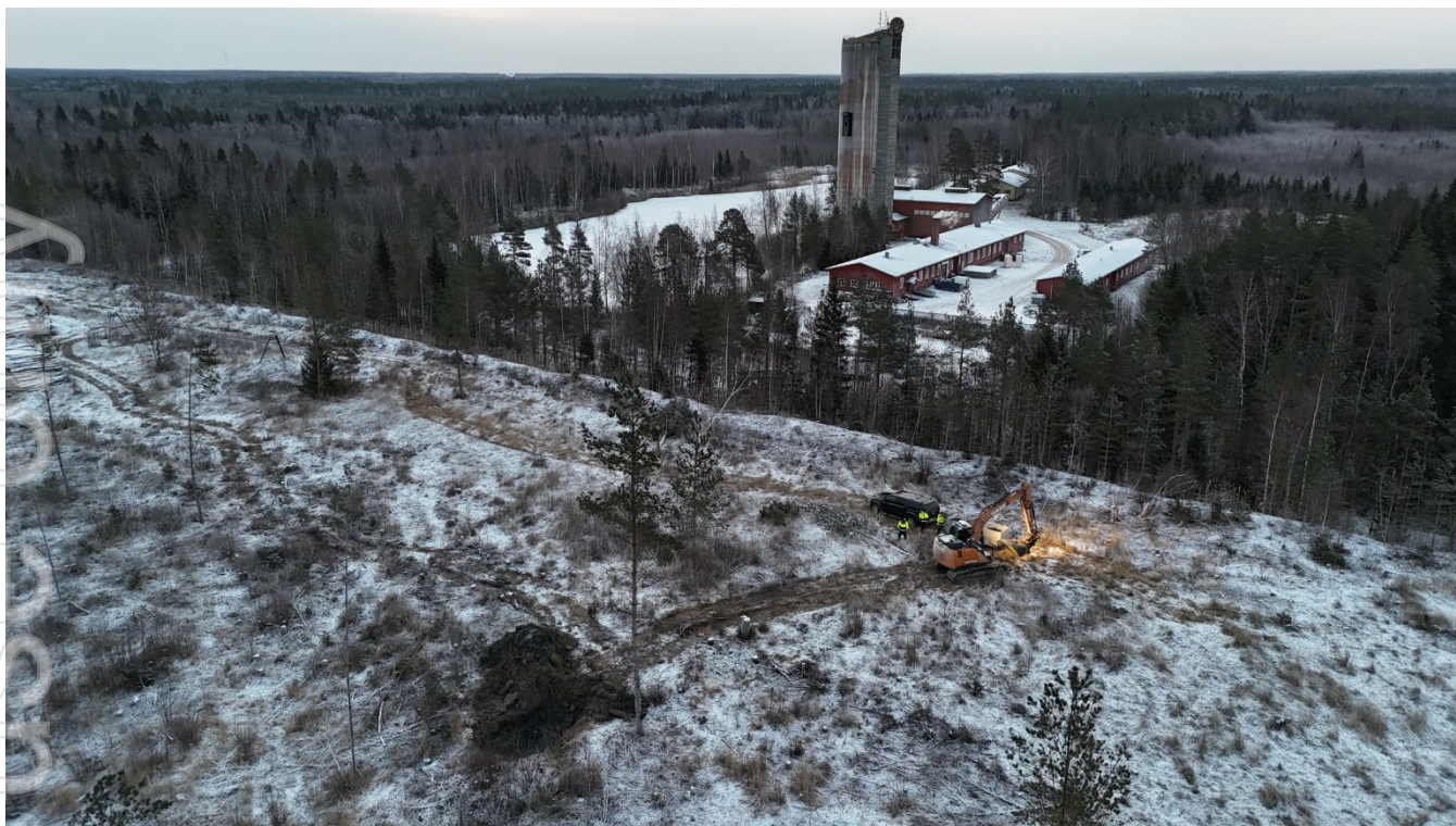
Collection of 3-tonne bulk sample from Korsnäs TSF to support REMHub pilot plant runs at the University of Oulu.
