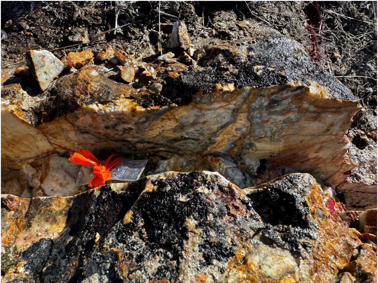
Figure 14. Sawn Channel sample showing epithermal textures within the vein. Sample ID CC278, returning 1.6m @ 333g/t AgEq (136g/t Ag & 2.4g/t Au) or 4.0g/t AuEq. 4 Looking North.
