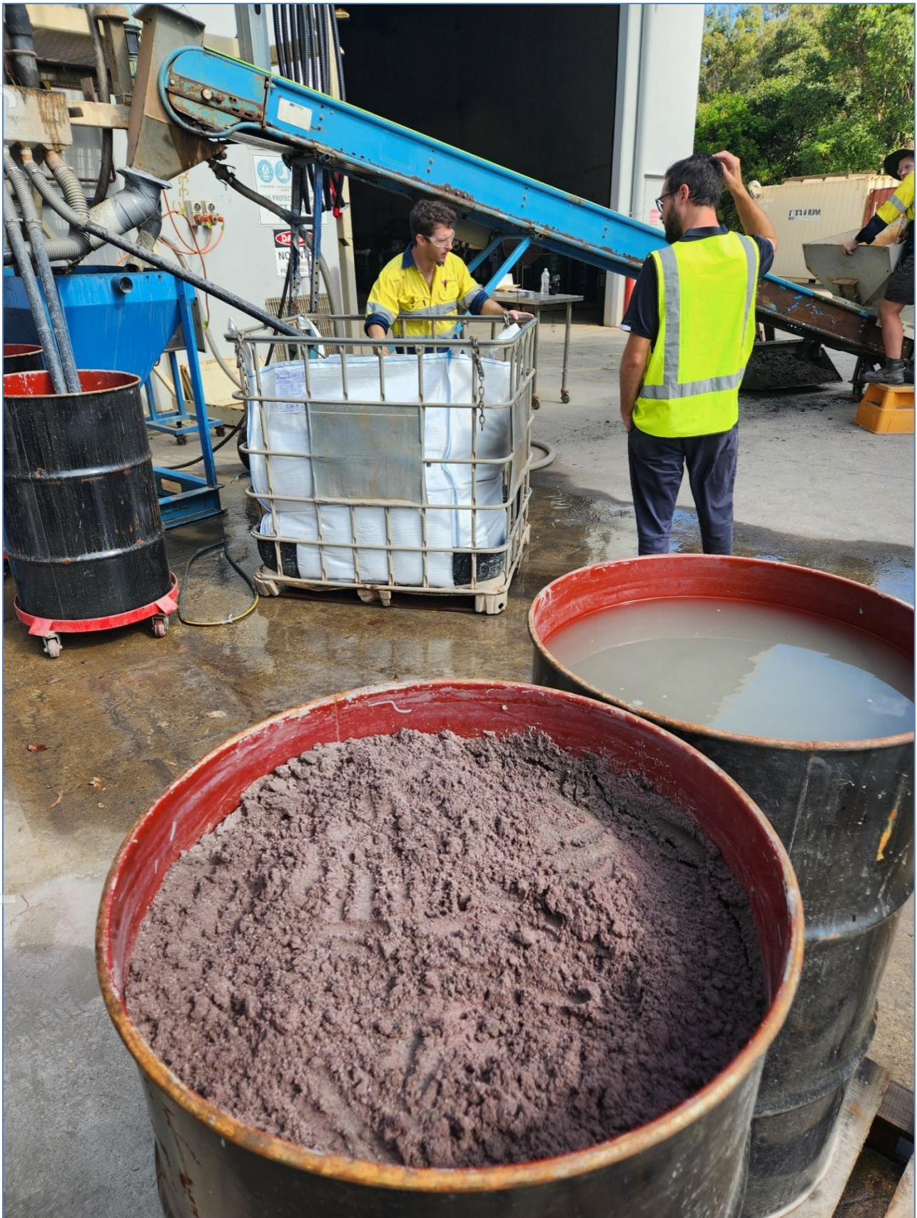
Figure 7 – IHC processing Kanmantoo Mine bulk tailings Sample in May-June 2025. Garnet Concentrate visible in drum.
