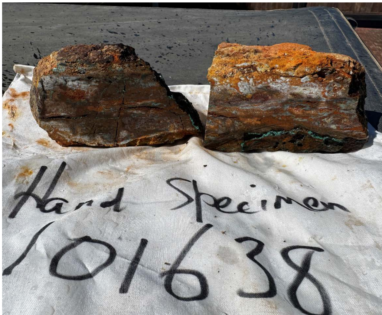
Figure 16. A photo of a sawn specimen collected from outcrop rock chip SampNo 101638 within the Cardross Mining Lease, assaying 6.84 g/t Au, 330 g/t Ag, 7.72% Cu (Figs. 2 and 5, Table 1). The significance of similar high grade copper, gold and silver lodes seen throughout Cardross are being evaluated for future resource estimation considerations.
