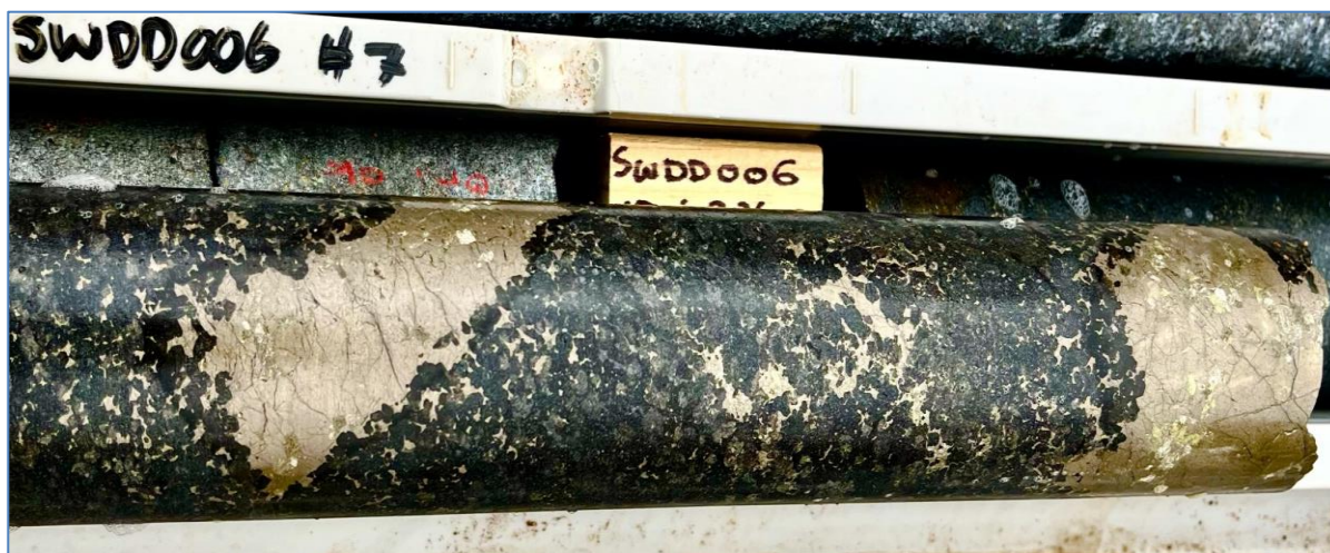
Figure 5. Drill core from hole SWDD006 (226.55 – 226.85 m) showing net-textured to semi-massive magmatic sulfide mineralisation composed predominantly of pyrrhotite, pentlandite, and chalcopyrite (refer ASX announcement dated 29 October 2025 for further details).
