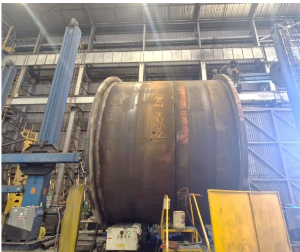
Figures 1 & 2: Components of the Kobada ball mill cast in the NCP factory - shell (LHS) and girth gear (RHS)
