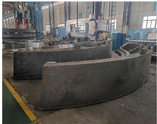
Figures 1 & 2: Components of the Kobada ball mill cast in the NCP factory - shell (LHS) and girth gear (RHS)
