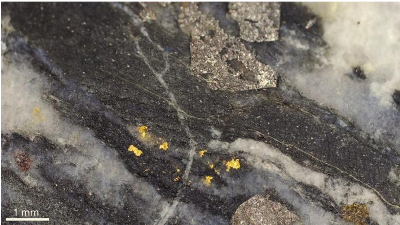
Figure 4. Microscope image of core from 25NED007 containing visible gold and pyrite at Comstock (St Arnaud) 14
